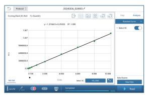
**02** Simply lay out two standard points to complete curve calibration
