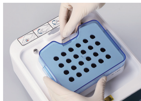
Figure: Toggle handle to replace block
